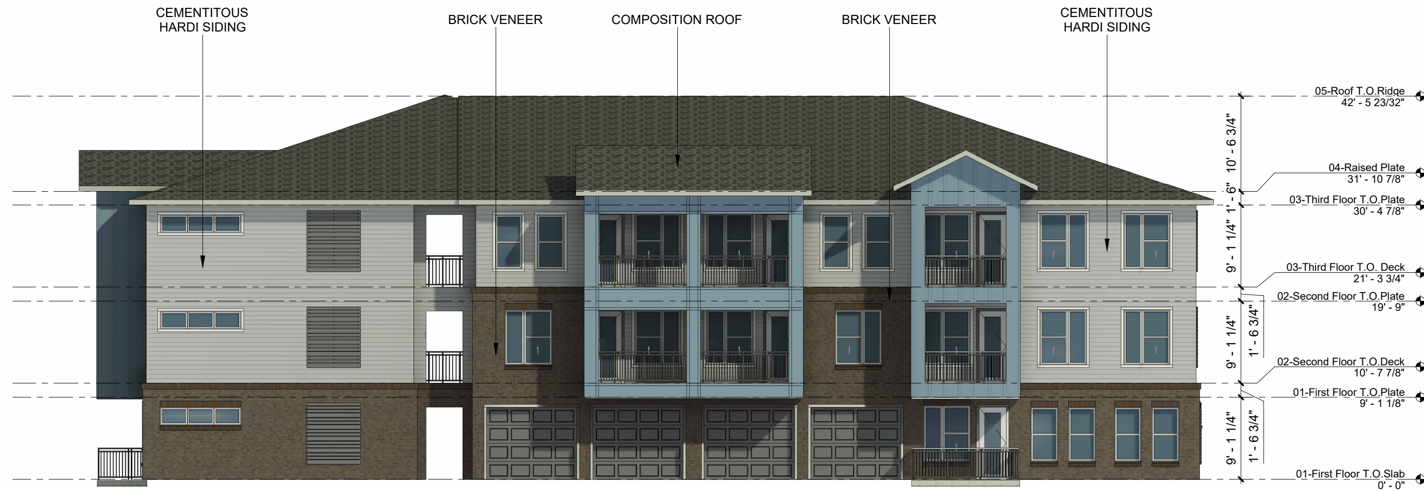
1 BLDG. #3 WEST ELEVATION 3/32" = 1'-0"
