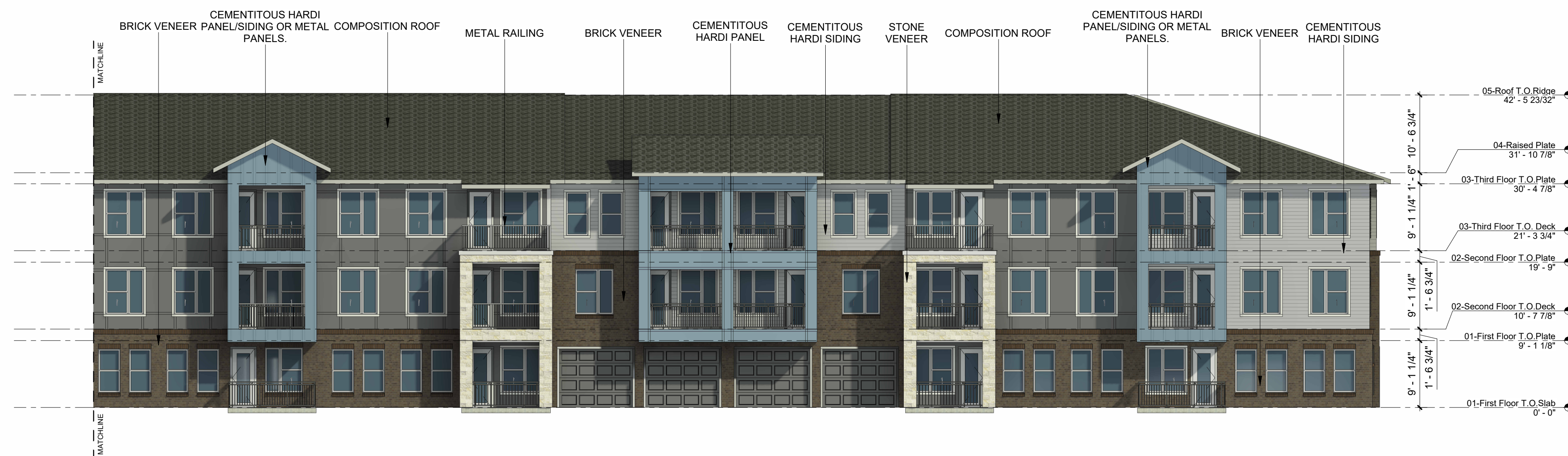
4 BLDG. #3 NORTH ELEVATION CONT'D. 3/32" = 1'-0"
