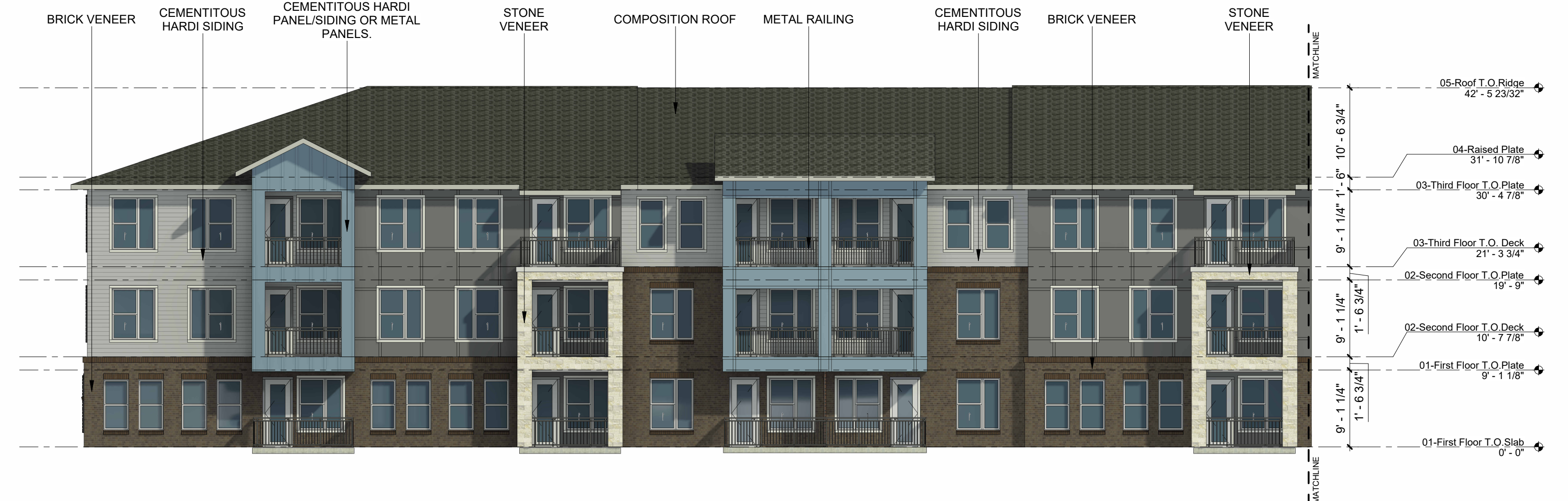
3 BLDG. #3 NORTH ELEVATION 3/32" = 1'-0"
