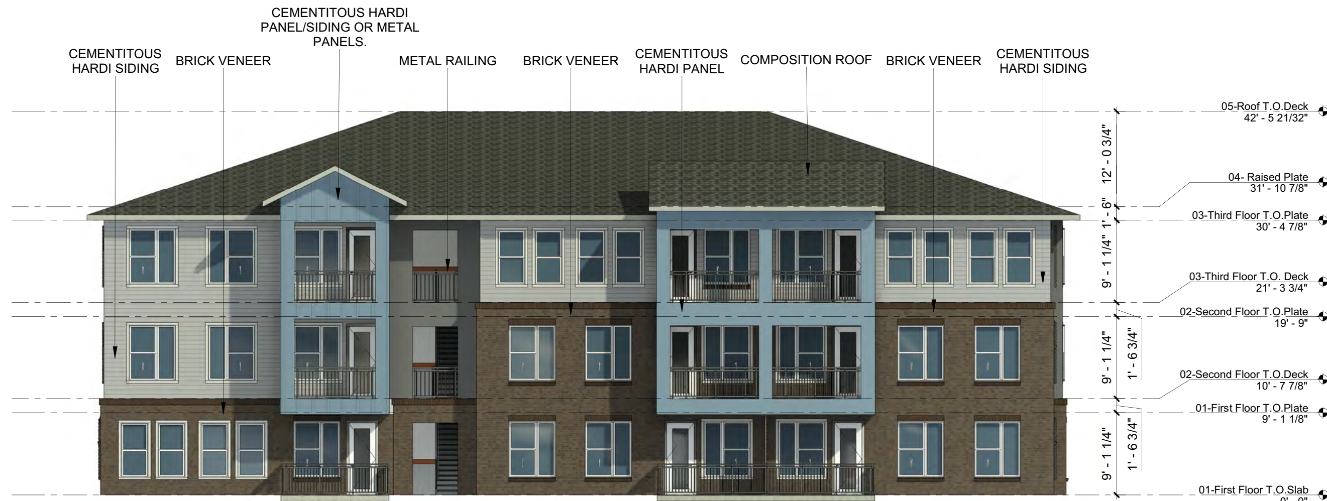
3 BLDG. #2 WEST ELEVATION 3/32" = 1'-0"
