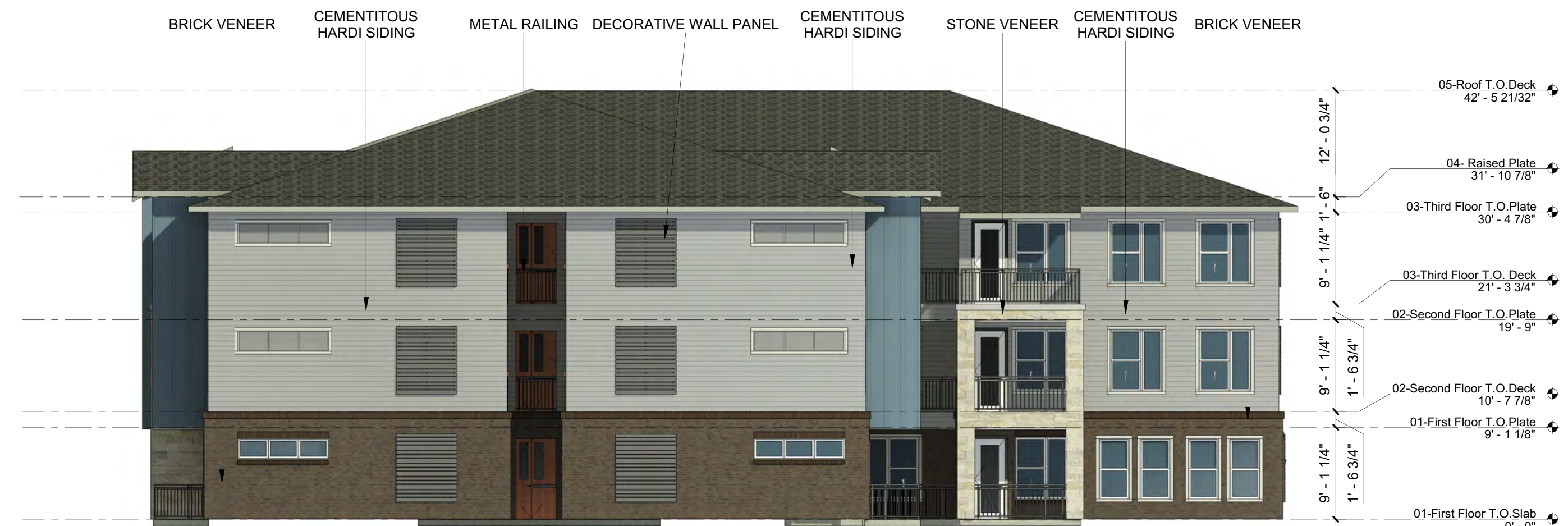
4 BLDG. #2 EAST ELEVATION 3/32" = 1'-0"
