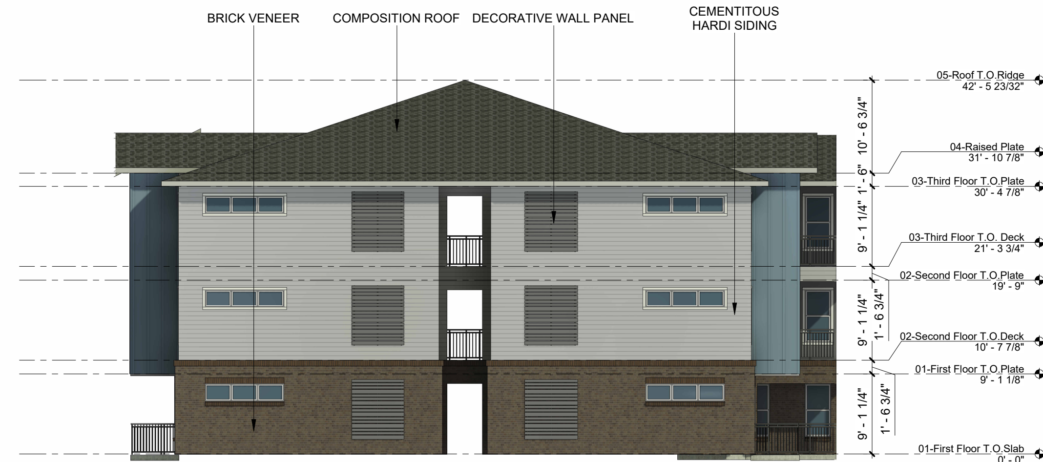
2 BLDG. #3 SOUTH END ELEVATION 3/32" = 1'-0"
