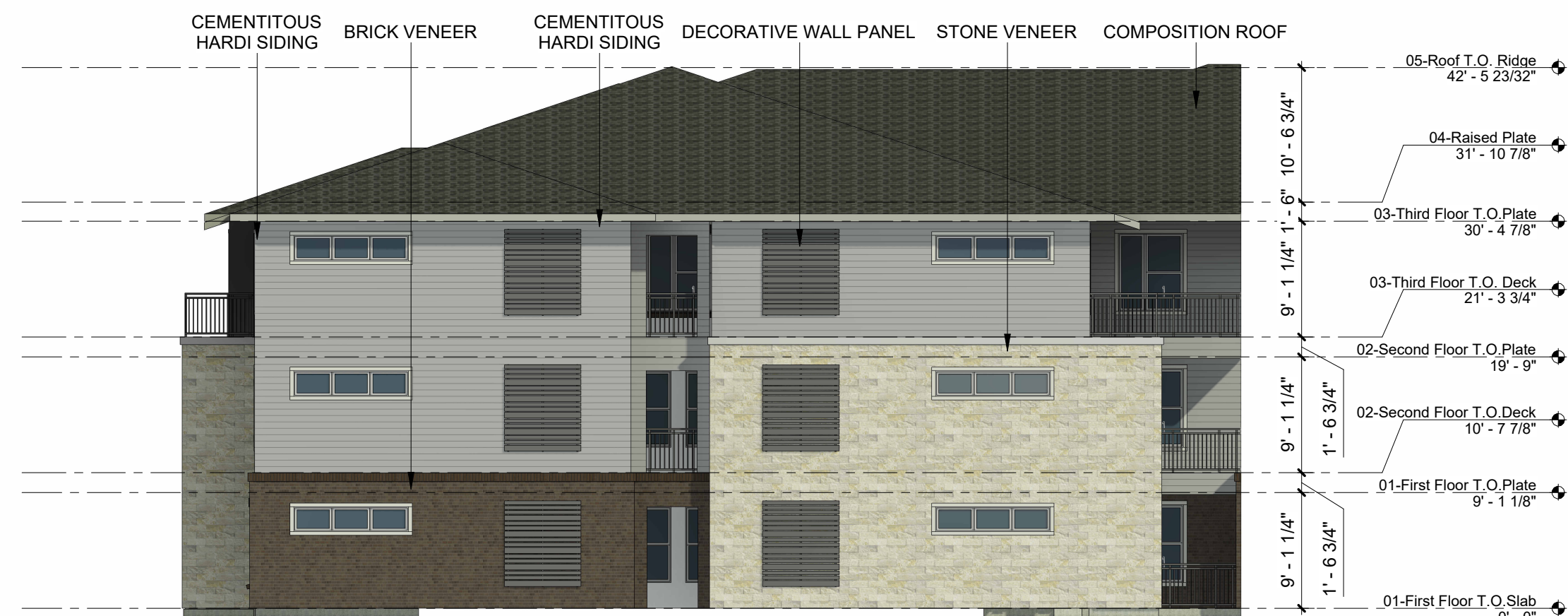
4 BLDG. #1 EAST END ELEVATION 3/32" = 1'-0"
