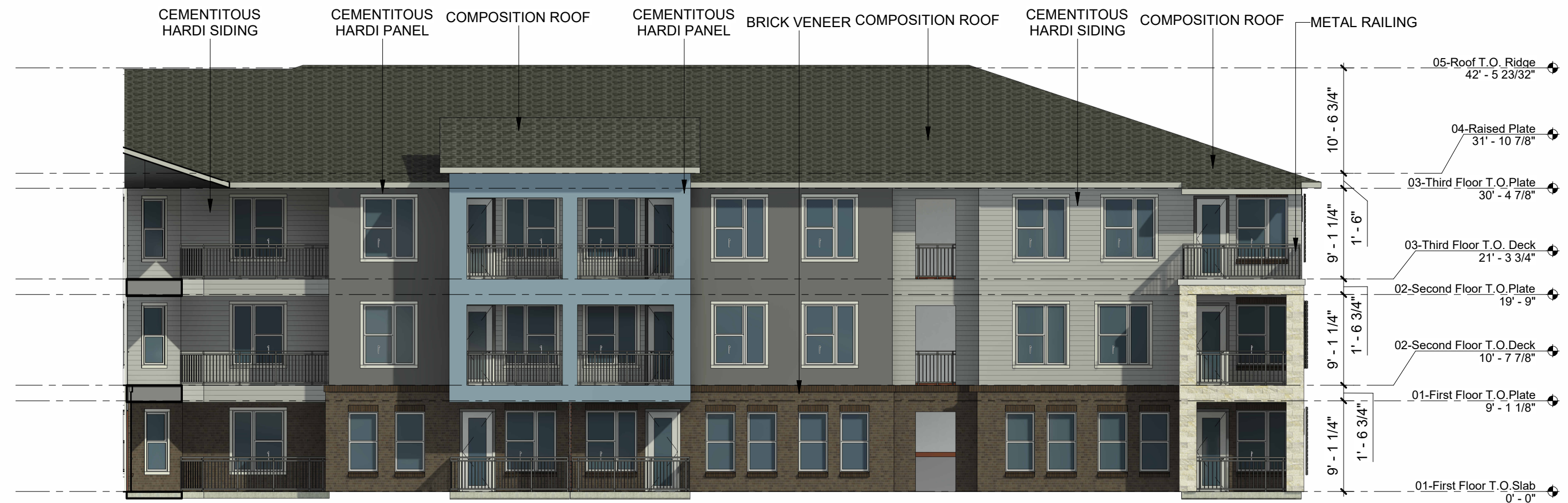
3 BLDG. #1 EAST ELEVATION 3/32" = 1'-0"
