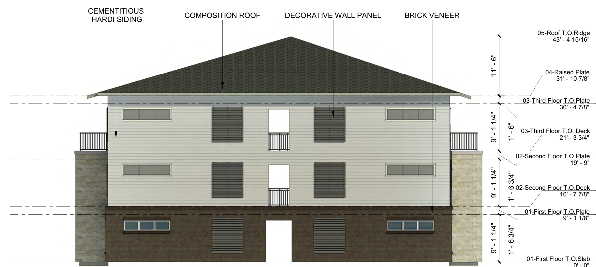
4 BLDG. #4 - EAST ELEVATION 3/32" = 1'-0"
