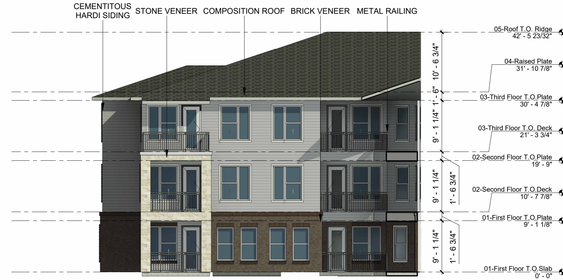
6 BLDG. #1 NORTH CORNER ELEVATION 3/32" = 1'-0"
